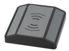
The fully potted RFID mounting reader MCR (Multi Card Reader) LEGIC was developed for easy installation on 55 mm switchbox or for surface mounting (frame supplied).
