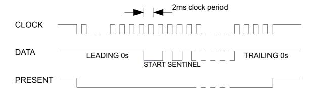
Each character is 5 bits long. The first four bits are the hex digit (0-F) least significant bit first. The fifth bit is the odd parity bit. A 0 is represented by a high level on the DATA wire and a 1 is represented by a low level on the DATA wire. Data is set up on the falling edge of the clock and is stable on the rising edge of the clock. The PRESENT output goes low for the duration of the transmission simulating the CARD PRESENT from a mag. card reader.
