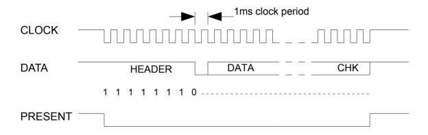
Data is set up on the falling edge of the clock and is stable on the rising edge of the clock.
